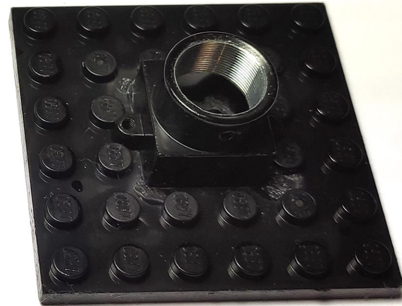
TREEYE M12 lens holder (alternative to the 3D printed adapter)
